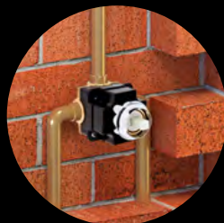
Installation of piping to the concealed part.
