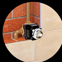
Plaster and ceramic tiles assembly.
